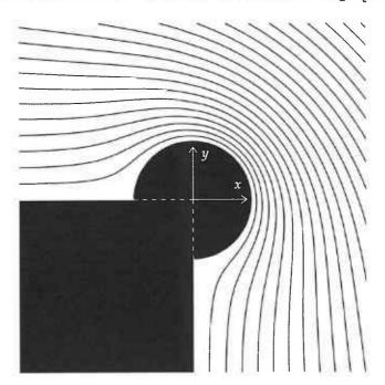
Consider a two-dimensional, steady, incompressible (density  $\rho$ ), inviscid, and irrotational flow around a square corner with a circular bump. The stream function  $\psi(r,\theta)$  is given by:
